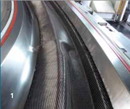
1 Carbon fiber preform in RTM mold.
